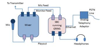
Figure 2: A radio station setup using GRINS: The single board computer (SBC) running GRINS is connected to the mixer, which is in turn connected to the transmitter. The Telephony adapter allows connecting the PSTN line to the SBC.
