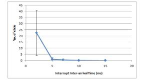
Figure 8: Impact of input and output interrupt inter-arrival times (IITs) on clicks in audio routing. Number of clicks reduce with increase in IITs.
