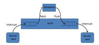
Figure 4: Audio transfer from line-in to line-out of a soundcard in GRINS
