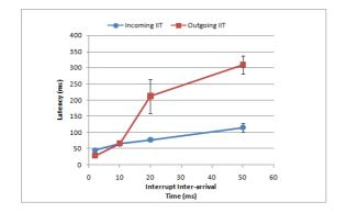
Figure 6: Impact of input and output interrupt inter-arrival times (IITs) on audio routing latency. Latency monotonously increases with increase in IITs.
